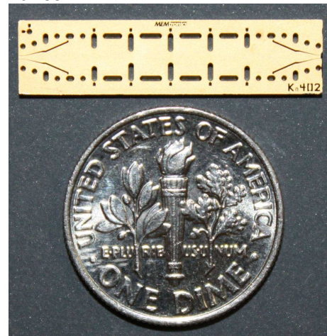
Figure 3. Ka-band substrate integrated filter developed as a demonstration platform for tunable filters.
